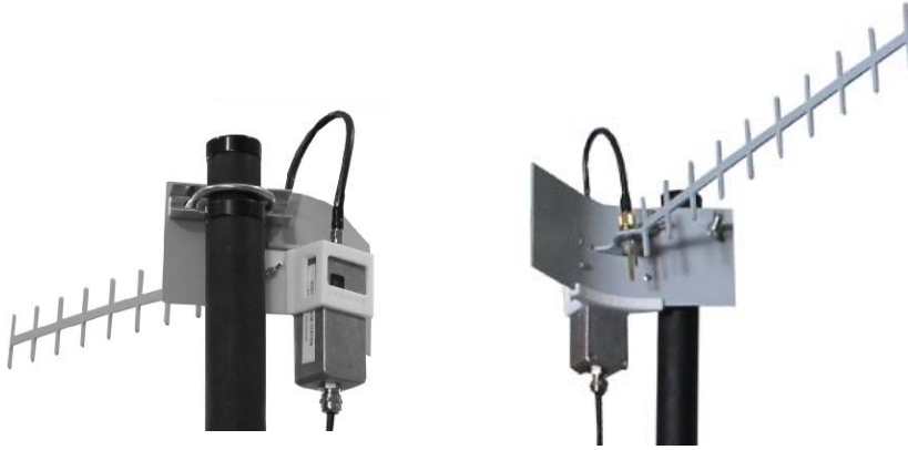
Figure 2 Assembly with directional antenna on mast.
