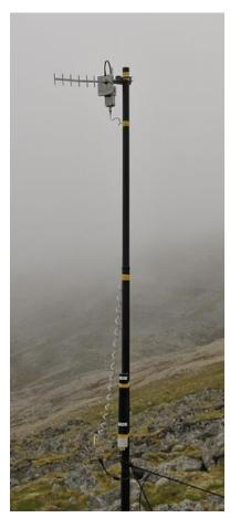
The unidirectional antenna can be used for loggers programming before attaching them to animals or when the base station is working in very short distance from the nest.
